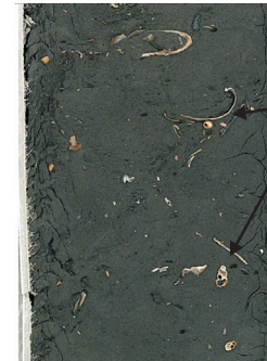
Facies 3 - Muddy silt with brackish water fauna. Occurrence of foraminifera, calcareous coccoliths and dinoflagellata tests.
